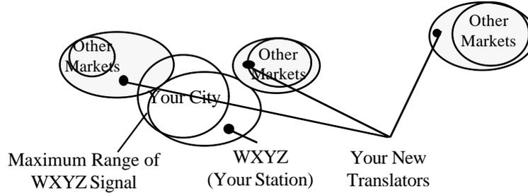
The FM Translator rebroadcasts signals from an existing FM radio station to areas that have unsatisfactory reception of the original station. Translators provide an excellent means of extending the broadcast range of the FM station.
