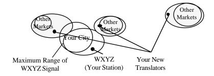
The FM Translator rebroadcasts signals from an existing FM radio station to areas that have unsatisfactory reception of the original station. Translators provide an excellent means of extending the broadcast range of the FM station.
